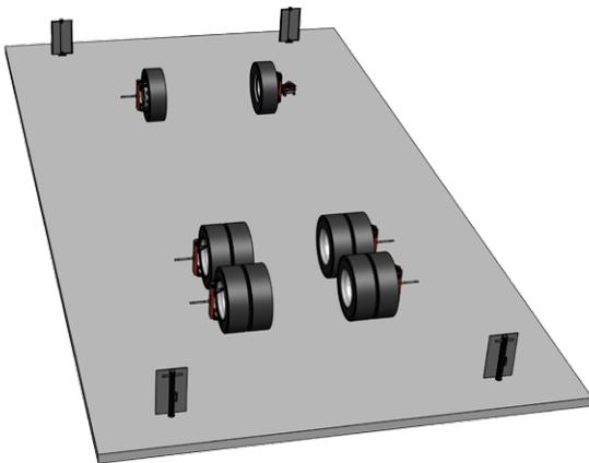
For the purpose of fast diagnostics and wheel alignment, the JOSA i-track target scales can be mounted on a dedicated floor area with a surface up to 22 meters in length, and about 4 meters in width.
