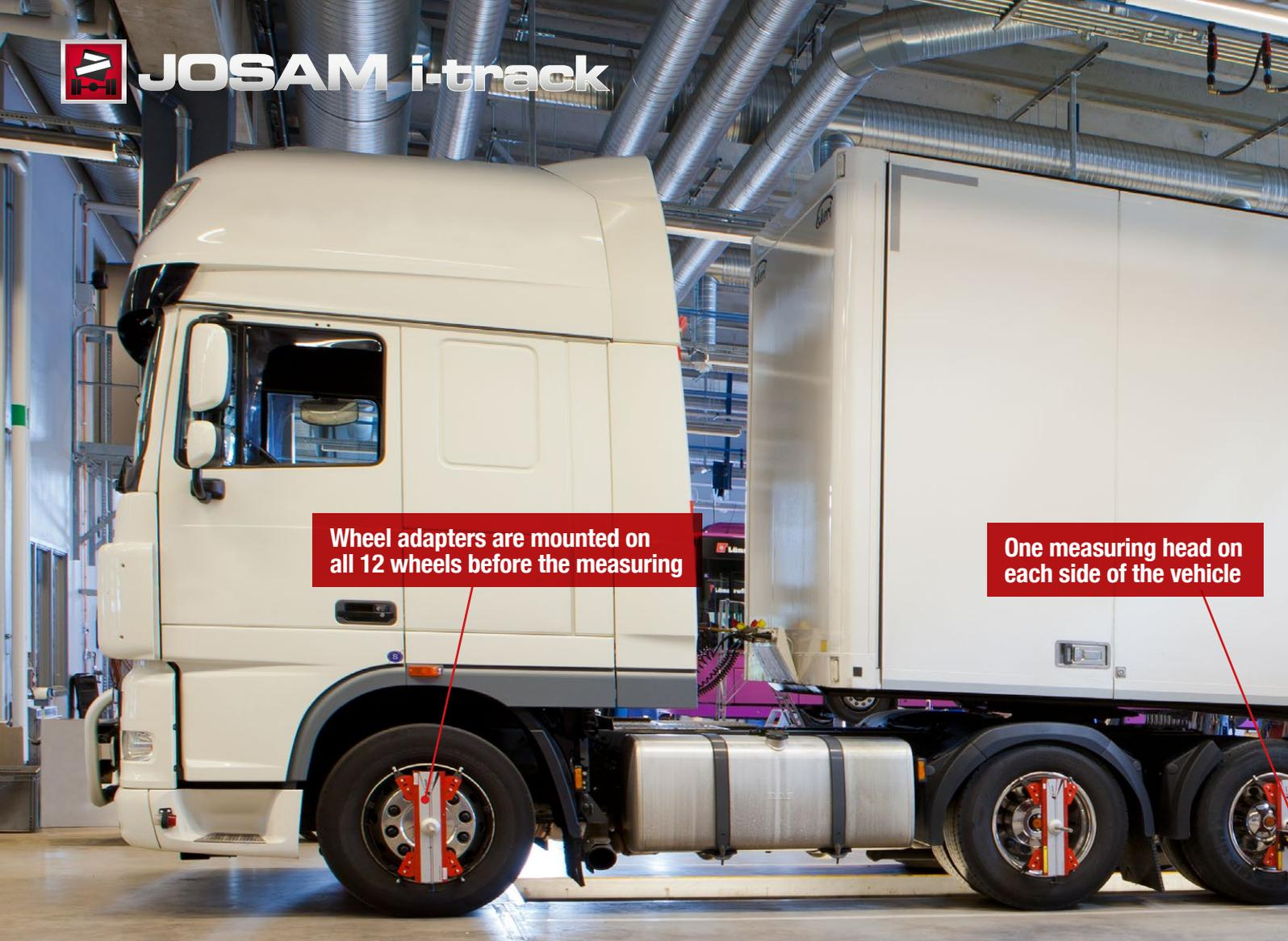
**Wheel adapters are mounted on all 12 wheels before the measuring**
