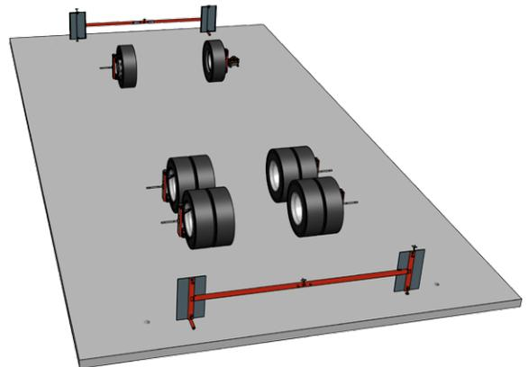
Adding flexibility, a mobile alternative is available so target scales can be moved to different locations. With this option, no floor drilling is needed. A fast and easy setup thanks to software guidelines and a perfect solution for multi bay operations and mobile units.
