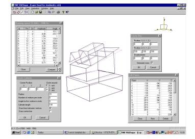
With the animation program Vibshape you can "understand" how a machine vibrates and what measures should be taken.
