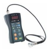
The VIBER X1™ portable Vibrometer consist of carrying bag, a vibration transducer with magnet support extension tip, charger and rechargeable batteries. The range can be set by adjustable filters from 2 to max frequency 16 000 Hz. It measures Bearing condition and vibration in velocity (mm/s RMS).
