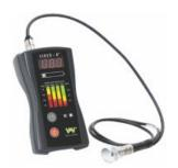
The VIBER-A+™, portable Vibrometer consists of soft carrying bag, a vibration transducer with magnet support. It measures Bearing condition and vibration in velocity (mm/s RMS) in two different versions, with frequency ranges 2 Hz or 10 Hz, 1000 Hz or 16 000 Hz. Tool for every engineers toolbox.
