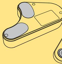
Magnetic reference surface on both transmitter and detector for easy attachment to the sheaves.
