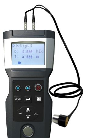
operating principles as SONAR it is capable of measuring the thickness of various materials with accuracy as high as 0.001 millimeters, or 0.0001inches. It is adapted to measure the thickness of good conductor for ultrasonic, such as metal (steel, cast iron, aluminum, copper), plastic, ceramic, glass, glass fiber and so on
