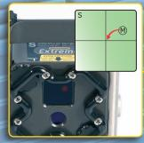
Electronic targets for adjustment of the laser beams to the detector centre.
