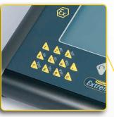
Connectors well protected against external damage.
