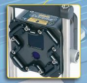
Smooth design, no pockets where dirt or liquid can collect. Makes it easy to keep the measuring unit clean. The impact-absorbing frame also functions as a safety cover for the detector surface.
