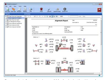
Screenshot from the Laser AM plugin in the Homebase software platform. The report sheet can be printed or saved as a PDF.
