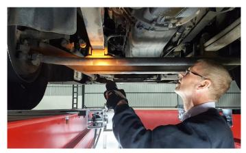
Before measuring wheel angles, the play detectors are used to check for worn parts.
