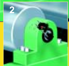
Parallelism measurement of rolls. (Detector with the magnet base on the roll shaft end.)
