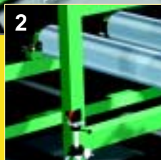
Parallelism measurement of rolls. (detector with the sliding bracket placed on the roll surface.)
